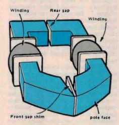
Figure 3. A typical record/replay head.
