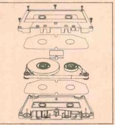
The patented BASF Security Mechanism (SM) prevents scrambling of tape and guides the tape smoothly within the cassette. A large strong window gives clear visibility to the best BASF ferro super I tape yet.
