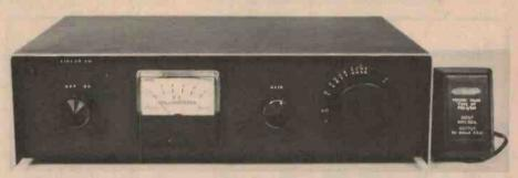
The tuner is housed in a simple, yet attractive, case. A plugpack is used to power the unit.
