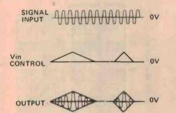
Figure 2. Illustrating the operation of the voltage controlled amplifier shown in Figure 1.
