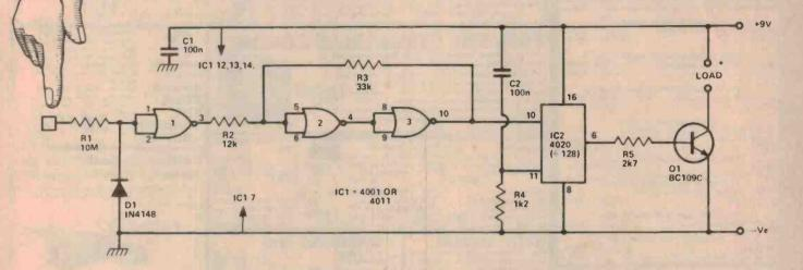
THIS TOUCH SWITCH is designed to provide on/off switching for 9 V battery operated equipment having a current consumption of up to 100 mA. It has a single touch contact which is briefly touched in order to change from on to off or vice versa. The circuit is operated by stray pick-up of mains hum which is coupled to the input of Gate 1 (which, like the other three gates employed in the unit, is connected to act as an inverter) via R1 when the input contact is touched.
