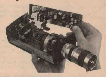
All the electronics for a new closed circuit TV camera are on a single printed circuit board.
