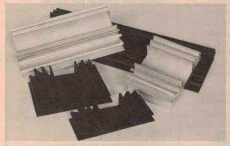
This heatslink, made locally by Rod Irving Electronics, is available in a variety of lengths, both anodised and unanodised. It measures 105 mm wide overall and the centre section is 35 mm wide by 5 mm thick. There are five fins on each side and a 220 mm length (anodised) has a thermal rating around 1°C/watt in free air. See Rod Irving Electronics, 425 High Street, Northcote Vic. 3070. (03)489-8131.
