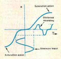
Figure 6. Distorted recording results from nonlinear tape transfer characteristic.
