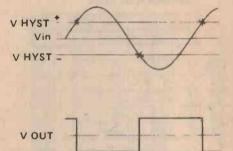
Figure 7. How the Schmitt trigger of Figure 6 works.
