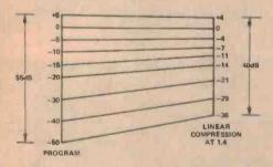
Figure 1. How linear compression reduces the dynamic range of programme material other. The 3BX continuously varies each of them, in response to the overall sound 'envelope'.
