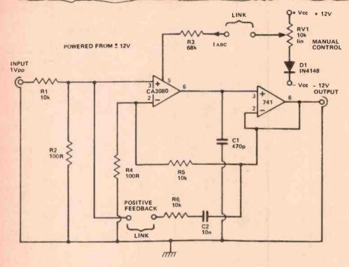
When this resistor is varied, the break frequency of the filter also varies.
