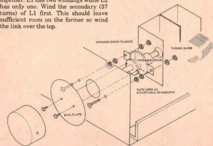
EXPLODED DIAGRAM OF VERNIER DRIVE AND DIAL ASSEMBLY
