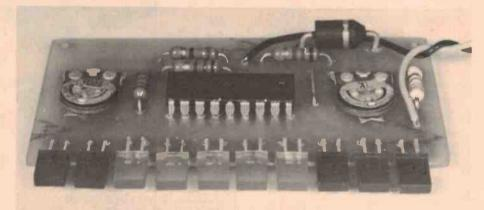
The completed voltmeter. LED1 (10.5 V) is on the right and LED10 (15.0 V) is at far left.
