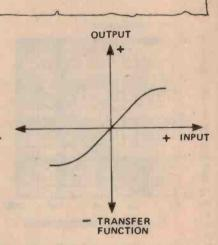
Figure 5. Transfer function of the Figure 3 circuit.
