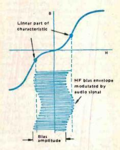
Figure 7. The distortion can be minimised by offsetting the audio signal onto a high frequency bias voltage.
