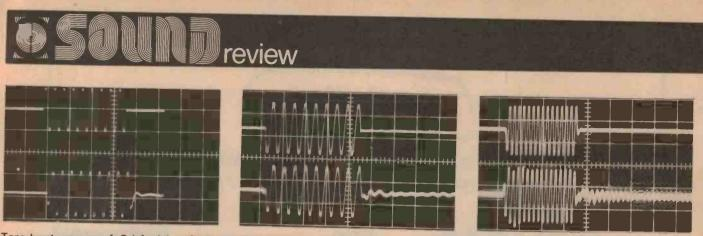
Tone burst response of Celef mini professional SM loudspeakers. Oscillograms taken at 90 dB steady state spl at 2m on axis. Left picture shows 100 Hz burst ('scope on 20 ms/div.). Centre picture shows 1 kHz burst (2 ms/div. on 'scope) and right shows 6.3 kHz burst (0.5 ms/div.).
