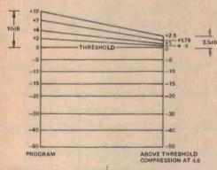
Figure 2. Above the threshold, compression has no effect on low level signals. When the signal exceeds the set threshold, the dynamic range is decreased. This is called 'above threshold compression' and allows higher compression ratios than linear compression.
