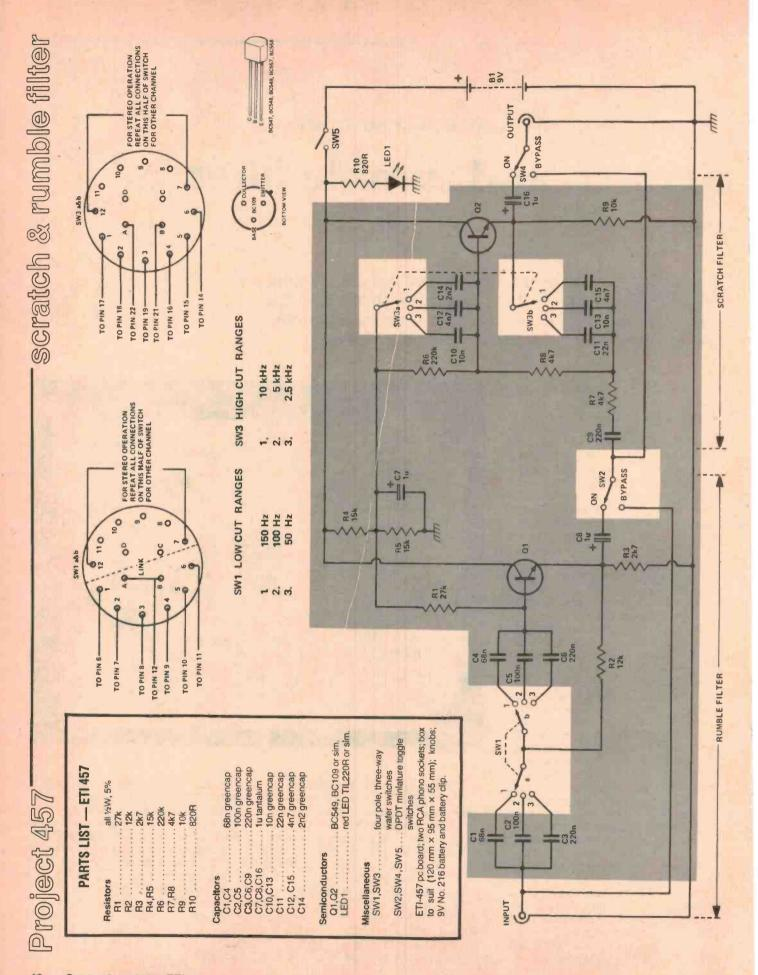
Figure 1 shows the block diagram of the mono version of the scratch and rumble filter. The input signal (from the turniable pick-up) is first fed through a high-pass filter, which rejects unwanted low-frequency rumble signals, and is then fed through a low-pass filter which rejects unwanted high-frequency scratch signals. Each filter can be bypassed via a simple switch if required, so the input signal can be passed through either one, both, or neither of the filters.
