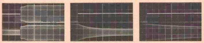
Dynamic characteristics. Expansion ratio – 1:1.5; Channel 1 input – 1 kHz tone burst; Channel 1 output is upper trace in each picture; Channel 2 input – 1 kHz steady state sinewave; Channel 2 output is lower trace in each picture. Left picture shows attack time ('scope on 50 ms/div.). Centre picture shows FAST release time ('scope on 200 ms/div.). Right picture shows SLOW release time ('scope on 200 ms/div.).
