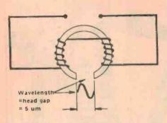
Figure 8. When the recorded wavelength equals the reptay head gap there is no flux linkage with the head core and consequently no output.
