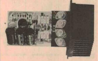
The same amplifier module as used in the complete amplifier. The 3002P.A. is based on the ETI 466 amplifier but with a redesigned P.C. board and much improved heatsink bracket. The module is designed to mount vertically in a 5¼" rack box. Complete kit includes P.C. board, all components and anodised heatsink bracket.
