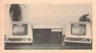
The new Opal microcomputer system, just released here by John F. Rose Computer Services, is believed to be the first S-100 microcomputer to incorporate an SA 1004 10M hard disk by Shugart.
