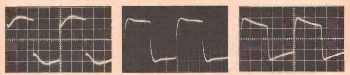
Square wave response of the dbx 3BX dynamic range enhancer: Expansion ratio - 1 : 1.5; Release time - FAST. Left picture taken with oscilloscope set at 2 ms/div., 100 Hz input. Centre picture has scope set at 0.2 ms/div., 1 kHz input. Right picture taken with 'scope on 20 us/div., 10 kHz input.
