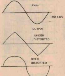
Figure 4. The output of the Figure 3 circuit should be adjusted (by RV1) to produce the waveform shown at top.
